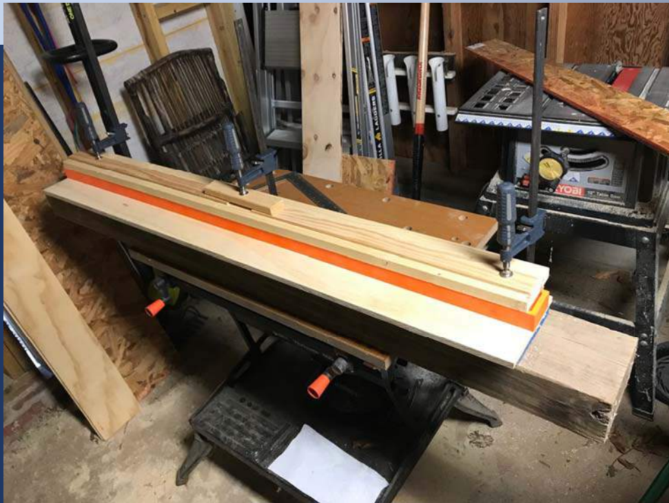
Clamped for routing
